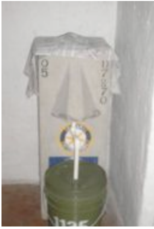
The locally-made Pure Water for the World concrete SSF design (Pure Water for the World)
